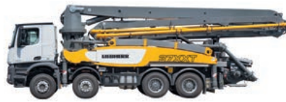
37 R4 XXT 36,8 m alcance vertical 32,8 m alcance horizontal
