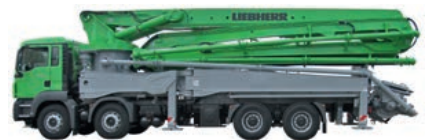
47 M5 ST 46,7 m alcance vertical 42,0 m alcance horizontal
