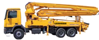
33 R4 ST 32,4 m alcance vertical 28,4 m alcance horizontal
