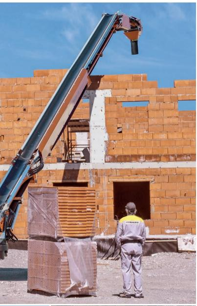
The Liebherr LTB conveyor can be attached to or removed from the truck mixer in a matter of minutes. This too makes its operation even more costeffective. Its closed structural elements and panels make the conveyor easy to clean quickly too.
