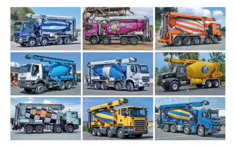
Truck mixers and conveyors from a single source, together with Liebherr's worldwide after-sales service, guarantee trouble-free operation. The Liebherr LTB conveyor can be installed on three- or four-axle vehicles. The customary mixer sizes are 7 m³, 8 m³ or 9 m³.
