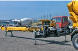
This is a most effective changeover system (option) that allows the Liebherr LTB conveyor to be attached and detached very quickly. There are other options too - please ask for details.
