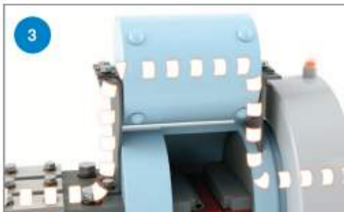
▲ The resultant arc voltage across this gap causes a transfer of the short-circuit current to a small, parallel current-limiting fuse.
