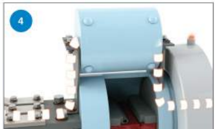
▲ The fuse melts and clears the circuit, as would a conventional current-limiting fuse. Current extinction occurs in the first half cycle, and limitation prior to the first peak.
