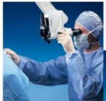
Standard working distances can be selected quickly and easily with the aid of click-stop settings at 250 mm (ear) and 400 mm (larynx).
