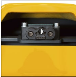
Electrical connection for trailers.
