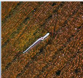
Laser-crystallized silicon on glass, EC EPIPLAN 10x/0.3
